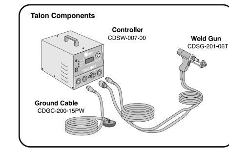
Remove the controller, cables and weld gun from the shipping packaging.
